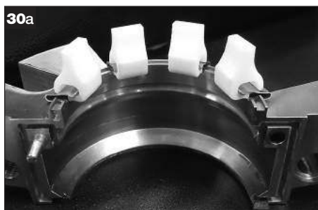
Spring lifter clips installed in gland halves.
