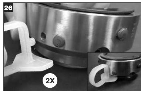
Install installation spacers on outside diameter of holder halves.
