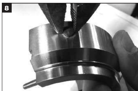
Remove used centering buttons from outside diameter of rotary holder.
