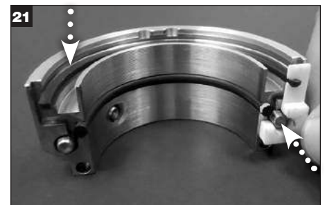
Install rotary holder shipping spacers in rotary holder halves to hold the rotary face O-Ring in place.
