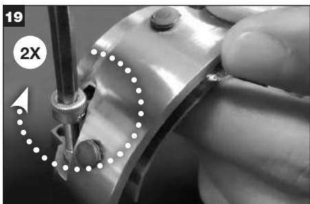
Lubricate threads with a recommended anti-seize compound and install holder cap screws in rotary holder half.
