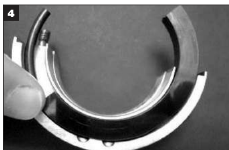
Remove used rotary face halves by pushing on end of face and sliding out of rotary holder half.
