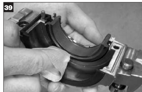
Clean stationary face halves with cleaning wipe to ensure there is no debris on face and at splits.
