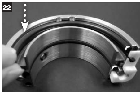
Apply a thin film of grease and install rotary face O-Ring halves in rotary holder halves.
