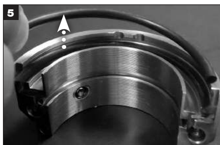
Remove used rotary face O-Ring halves.
